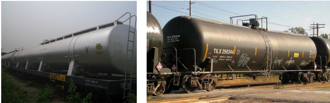
Figure II.6-5 Typical fuel tank wagon as operated by Nigerian railways (l), typical US tank wagon (r)
